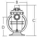
"SC" series swimming pool pump is designed for medium head installation in medium or domestic pool. 1.5 inch suction and discharge port with transparent lid. It operates at a low decibel and easy maintenance.
