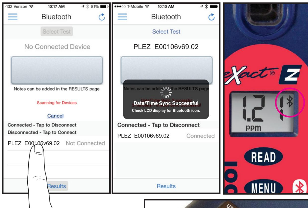
Refer to the back of your Pool eXact EZ to determine the serial number for your device. This will also be the name for the Bluetooth® connection.
