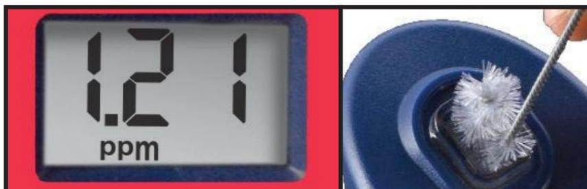
**Important!** Do not empty the CELL from **FREE CHLORINE TEST** if you are also testing for Combined Chlorine. You will need the sample.
