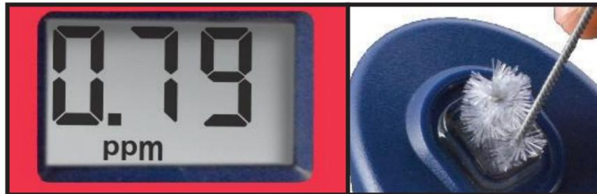
DPD will stain the CELL wall if allowed to remain in the CELL. To remove staining, rinse cell thoroughly and fill with water then add two (2) drops of bleach (5-8%) and clean with brush until stain is removed. Caution: Avoid contact of bleach with eyes and clothing.
